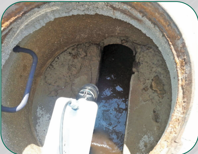
MICROFLOW-I IN A SEWERAGE NETWORK
